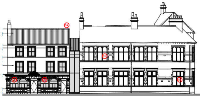
The relocated Earl de Grey and Castle Buildings, with the proposed link.
